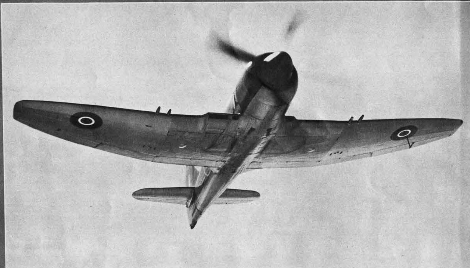
UNIQUE COOLING SYSTEM ON TEMPEST II BREAKS WING'S LEADING EDGE ON EITHER SIDE OF FUSELAGE. ARMAMENT CONSISTS OF FOUR 20-MM. CANNON
